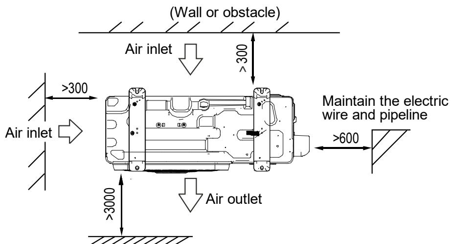
Figure 2-3.2: Multiple unit installation (unit: mm)
