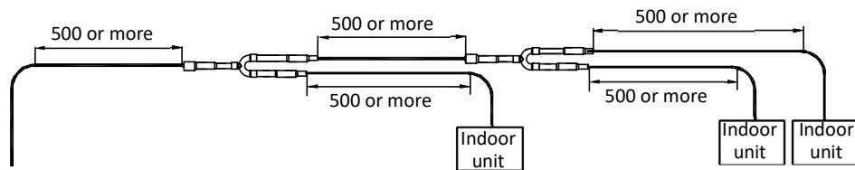
*Table 3-3.7: Indoor branch joint dimensions (unit: mm)*
