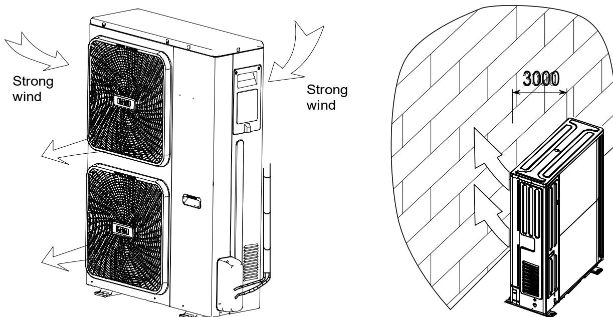
Figure 3-2.1: Single unit installation (unit: mm)
