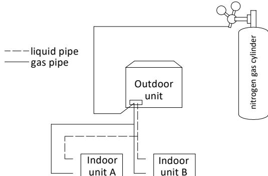
Figure 3-4.10: Pipe flushing sequence<sup>1</sup>
