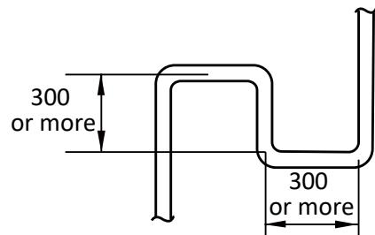
Figure 3-3.4: The first connecting method
