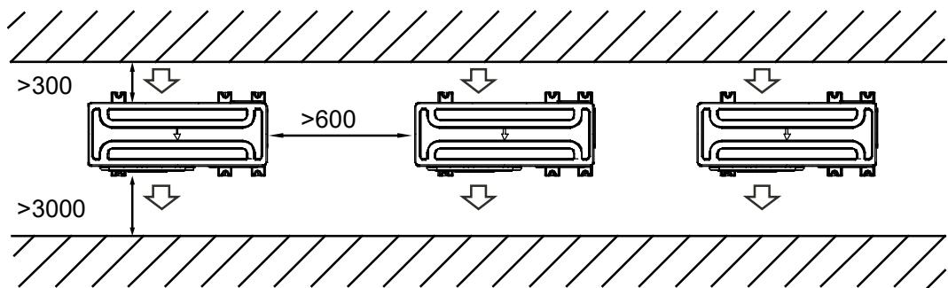
Figure 3-2.3: Parallel connection for the front with rear sides (unit: mm)
