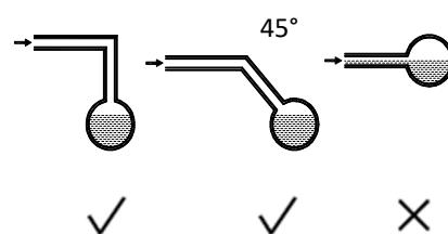
*Figure 3-5.4: Effect of insufficient drain piping support*
